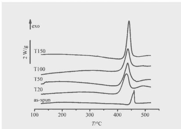
Fig. 3. Calorimetric curves obtained during heating at a heating rate of  $20^\circ\text{C min}^{-1}$  of HPT-processed and as-spun ribbons.
