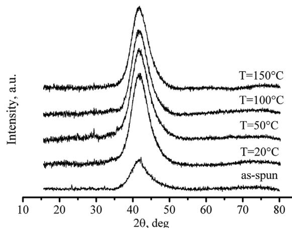
Fig. 1. The XRD patterns of the initial melt-spun  $\text{Ti}_{50}\text{Ni}_{25}\text{Cu}_{25}$  ribbon and melt-spun  $\text{Ti}_{50}\text{Ni}_{25}\text{Cu}_{25}$  alloy after HPT at different temperatures.
