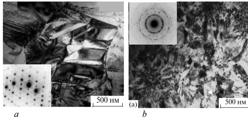
Fig. 4. (a) Bright-field TEM image and the corresponding SAED pattern for the MS  $Ti_{50}Ni_{25}Cu_{25}$  alloy after annealing at  $450^{\circ}C$  for 10 min; (b) bright-field image and the related SAED pattern (insert) for the MS  $Ti_{50}Ni_{25}Cu_{25}$  alloy subjected to HPT ( $T = 20^{\circ}C$ ) and subsequent annealing at  $450^{\circ}C$  for 10 min.
